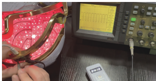
Figure 2: Mode 2 is pulse mode
